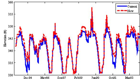
**Figure 2. The resultant lake elevation from the current and new rule curve**
