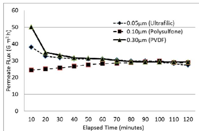
**Figure 3. Poultry processing wastewater permeate flux ( $G m^2 h$ ) values at 10 minute intervals for 3 membrane filters at 80 psi operating pressure**
