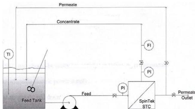
**Figure 1: Spintek Static Test Cell (STC) Membrane Filtration System (Source: <http://www.spintek.com/stc.htm>)**
