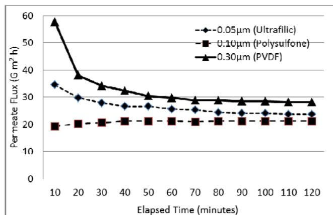
**Figure 2. Poultry processing wastewater permeate flux ( $G m^2 h$ ) values at 10 minute intervals for 3 membrane filters at 50 psi operating pressure**
